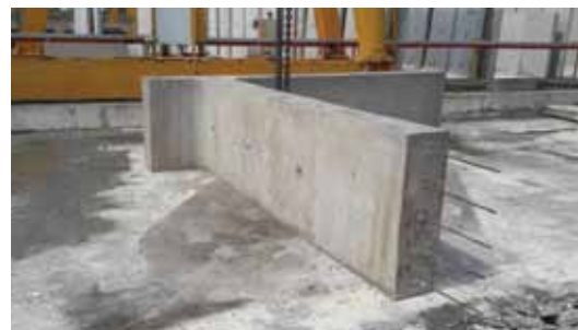
Picture: L-Wall with Precast Slap
